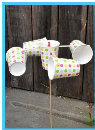
◀ A cup anemometer is commonly called a **Robinson anemometer**. It uses cup-like shapes to catch the wind, causing the device to spin. How many times it spins in a given time interval can tell you how fast the wind is moving.
